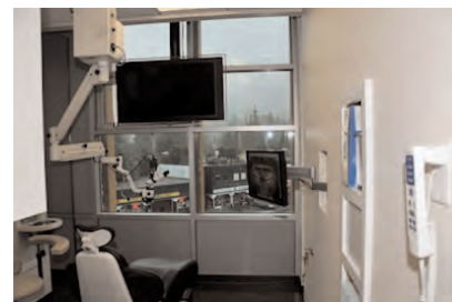
Fig 21 Forty-inch LCD monitor mounted at the foot of the chair to allow the clinician to properly and immediately assess framing, focus, and exposure of the images. In addition, the monitor can be used to playback images from the camera after the procedure for patient education.
