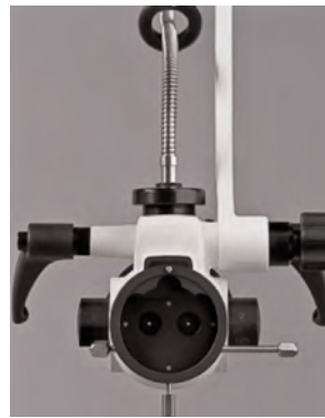
Fig 22 (left) Dual iris adapter situated between the magnification turret and oculars.
