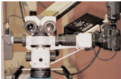
Fig 2 Original Global G6 microscope with strobe flash, Contax 35-mm slide camera on the right side, and one-chip analog video camera on the left side.
