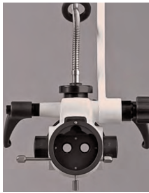
Fig 22 (left) Dual iris adapter situated between the magnification turret and oculars.
